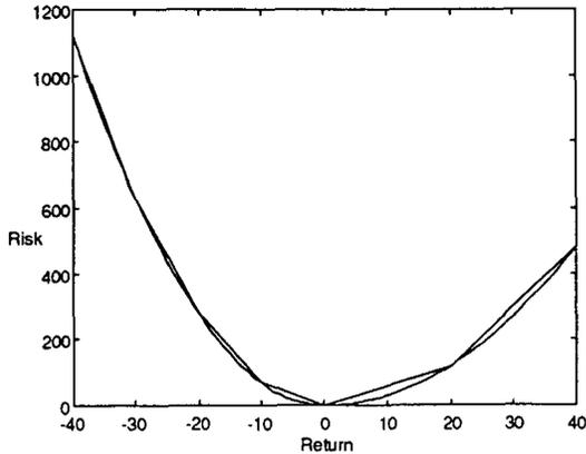
Fig-2. Converting a convex risk function  $N(0.7,0.3)$  into a piecewise linear format
