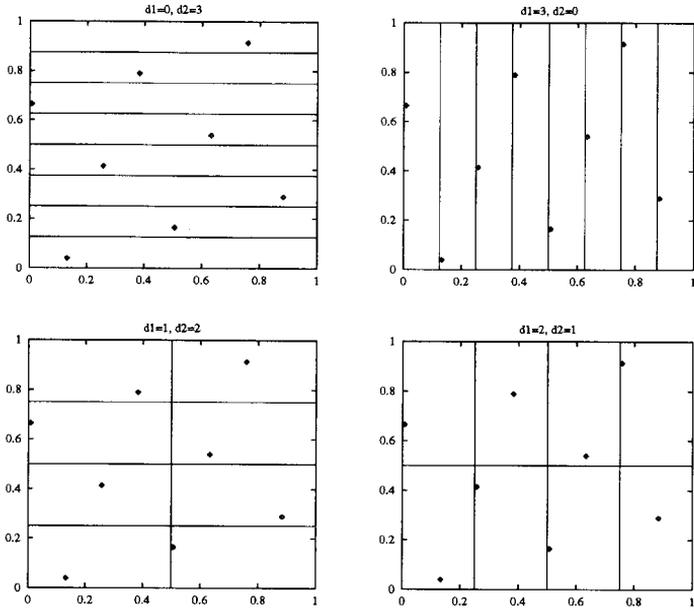
Figure 1: 4 Characterizations of Elementary Intervals for the First 8 Points
