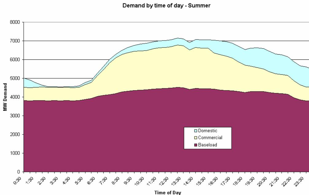
Summer days are characterised by a strong rise in demand during the middle of the day, driven by commercial airconditioning load. In recent times, this daytime peak has been extending well into the evening as domestic airconditioning load increases.
