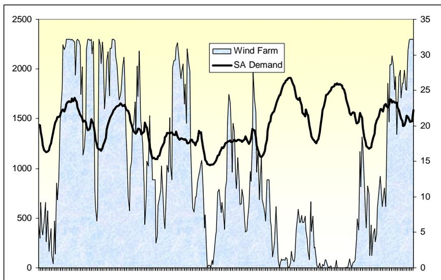
Wind is clearly intermittent, and further, wind generation output is not easily controlled: note the current Australia system sees large scale generator output centrally controlled through the dispatch and pricing system.
